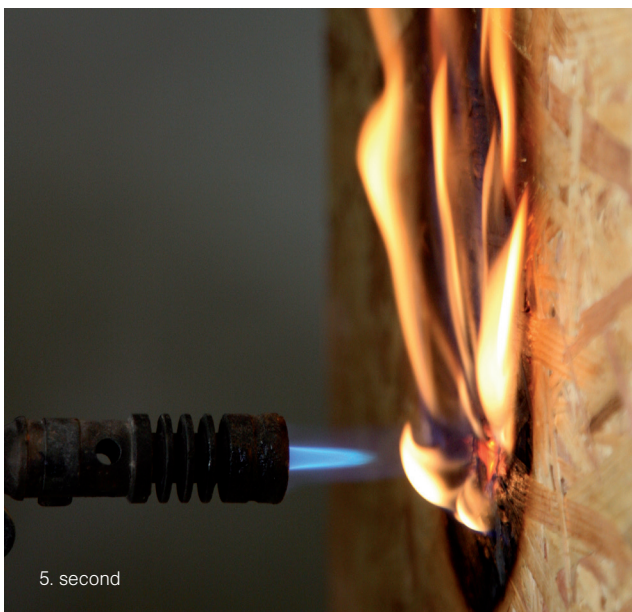
Picture No. 2.: Using OSB boards with Pyrotite® coating can extend the time to flashover from several minutes to a few tens of minutes.
