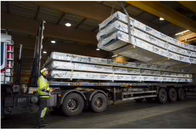
Figure 3.2. Loading LVL packages with an overhead crane for truck transport.
