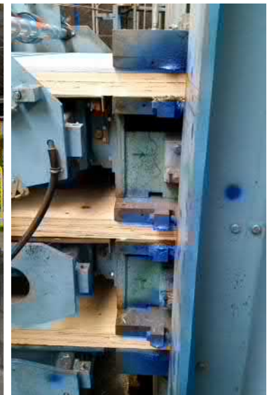
Figure 1.43. Feeding LVL billets into 3-level hot press.
