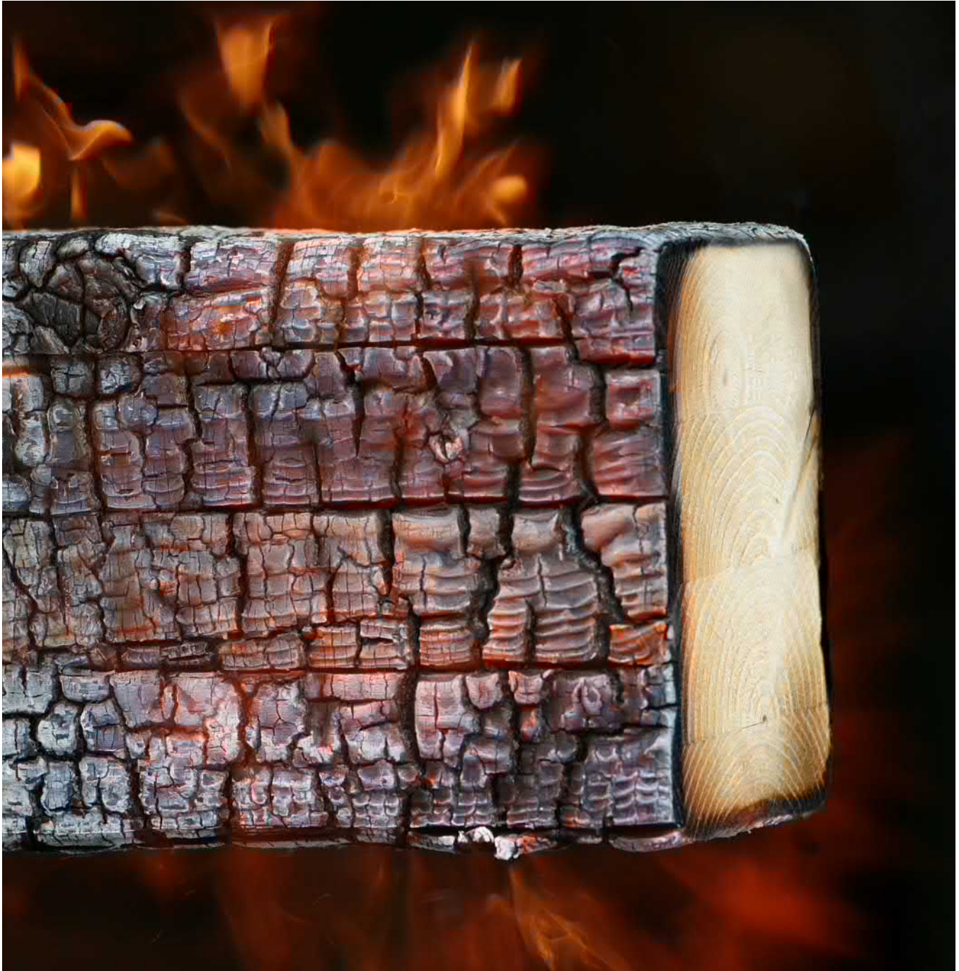
Figure 6.1. Charring of wood.
