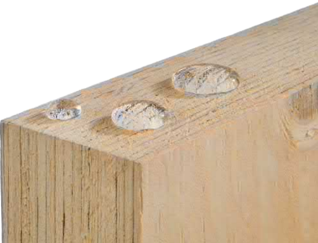
Figure 7.3. Moisture protection treatment on LVL beams.
